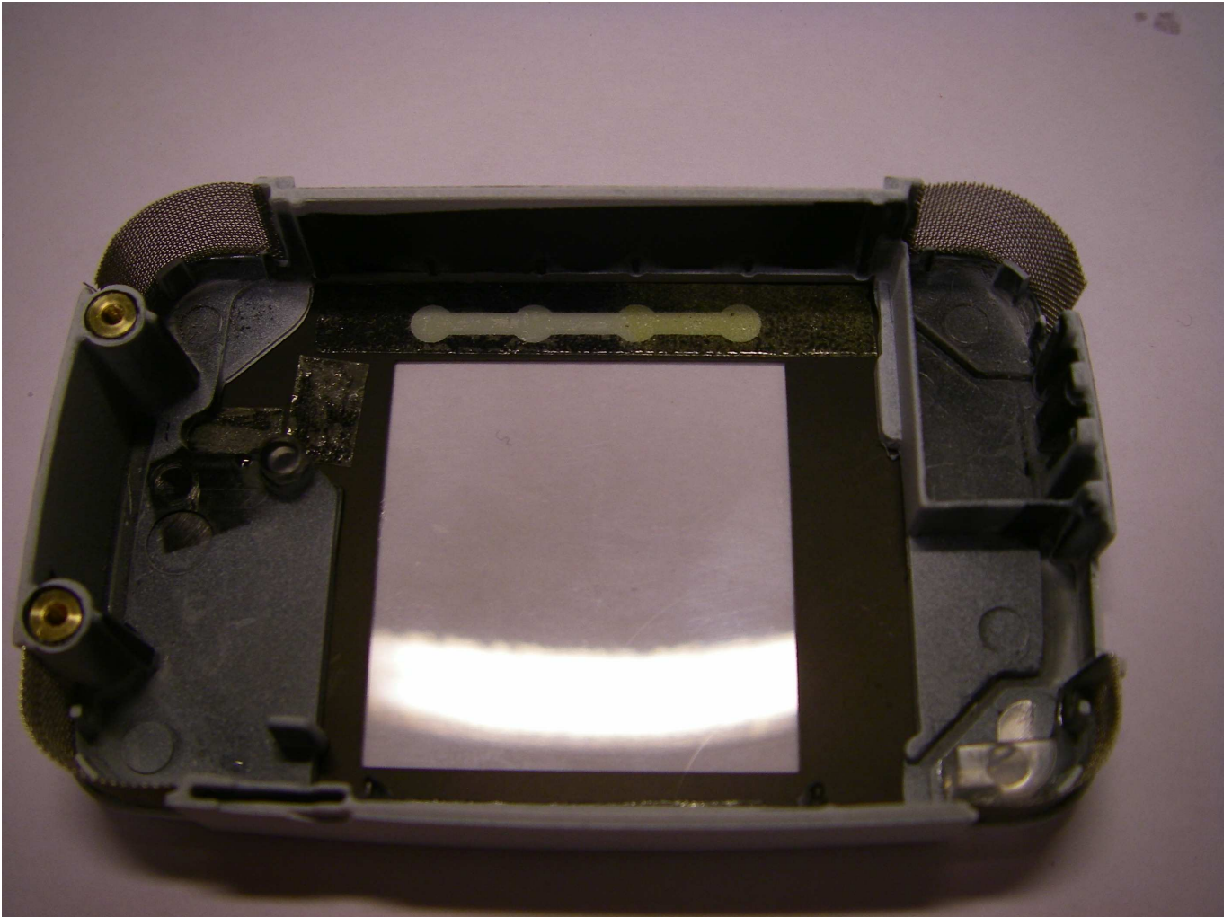
Figure 10 Attach the window to the top cover. Press firmly so the double sided tape will stick properly.
