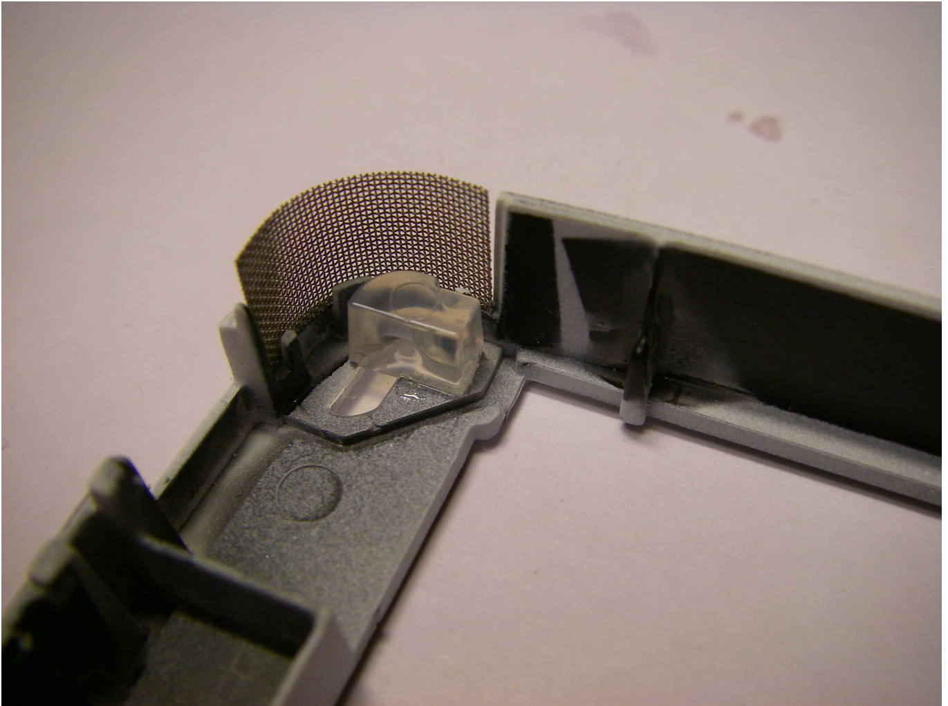
Figure 7 Detail of steel grid and light guide.
